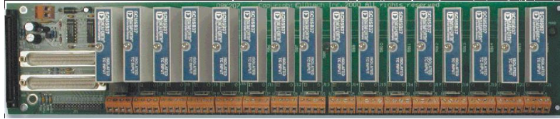
DBK207/CJC Carrier Board for 5B Compatible Modules
